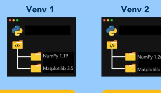
Venv operates independently, ensuring alterations to installed dependencies within one environment remain isolated from others and system-wide libraries. This isolation allows the creation of multiple virtual environments, each hosting its own Python versions and varying sets of libraries.
